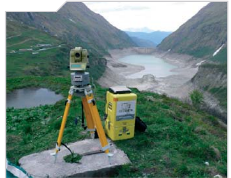
Calibration measurement for a hydro-power project
