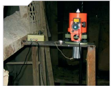
Schaft plumbing with precision optical plumb
