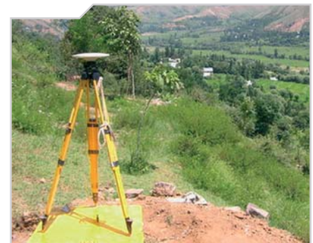
GPS-measurement for a tunnel network in India
