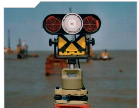
Offshore network measurement for galleries of a sewage water outfall project in Mumbai, India
