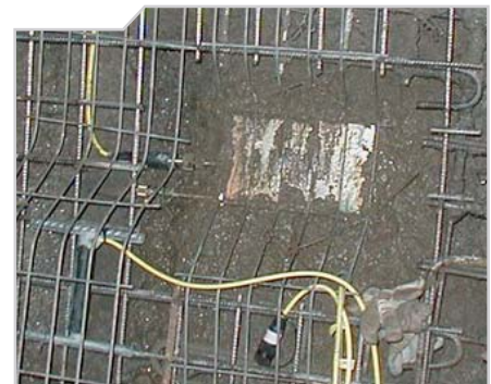
Pressure cell for determining the contact stress between ground and shotcrete-shell (in combination with strain meters)
