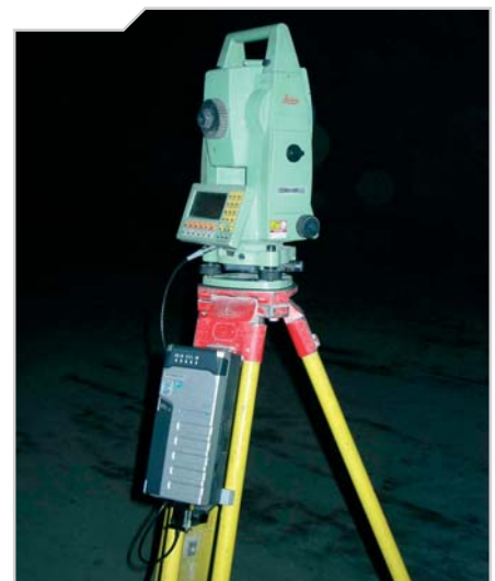
Totalstation with PC on tripod
